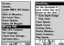
System Setup Menu (left) with Pop-up Help highlighted. The Pop-up Help message for the Sensitivity command (right).
